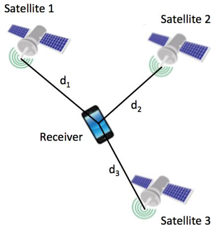
The distance to the first satellite defines a set of possible locations where the receiver could be – a circle (or a sphere in 3D) around the satellite. Each other satellite also defines a circle of possible locations. By
